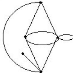
5. Let  $A$  and  $B$  be the respective circuit matrix and the incidence matrix (of a self loop free graph) whose columns are arranged using the same order of edges. Then every row of  $B$  is orthogonal to every row  $A$ . i.e  $A \cdot B^T = B \cdot A^T = 0 \pmod{2}$
